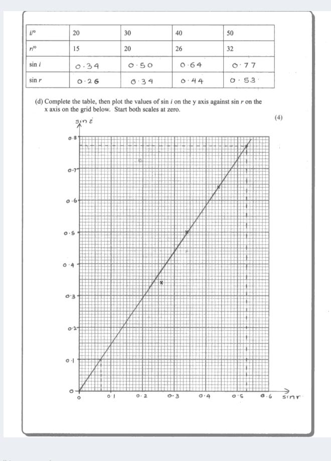
(e) Draw a line of best fit on your graph and explain why you think it should or should not go through the origin. (2) \* it should go through the origin. \* Because when the angle of incidence in O", ongle of refraction is also o' \* .'. sin 0' = 0 (f) Use your graph to determine the refractive index from air to glass. (2) refractive index · gradient of the graph.  $\frac{0\cdot 77 - 0\cdot 10}{0.53 - 0\cdot 17}$ - 1.46 - 1·s Refractive index =
